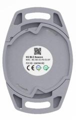
Default settings - 1 active slot, 1000ms ADV interval and 0 dBm Tx power
