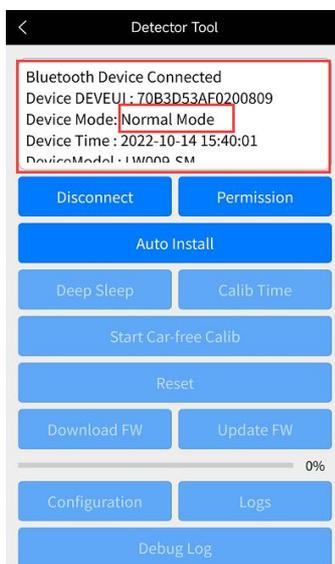
**Note:** make sure there are no vehicle and other metal material within 1 meter around the device or calibration will make error before “Auto Install”.
