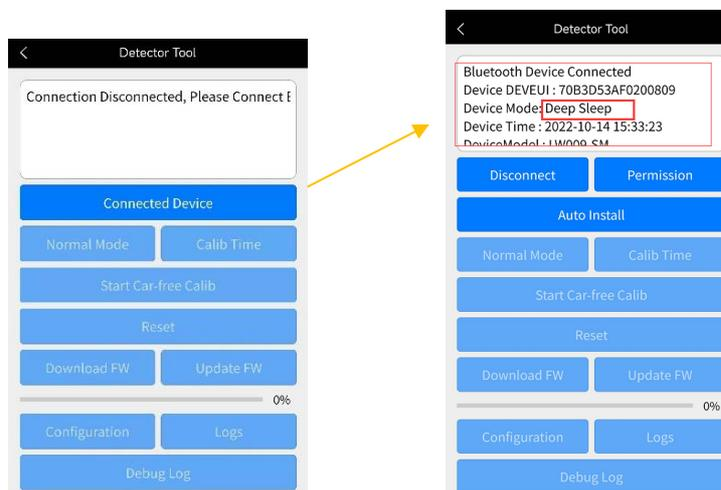
**Step 5:** Select “Auto Install”, the device will wake up and do the calibration automatically, the system time will be synchronized. The device mode will be Normal Mode.
